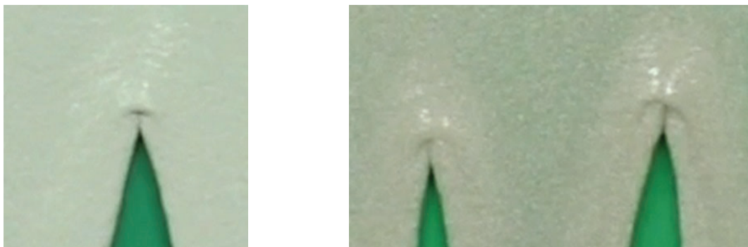
Figure 7. Two images of folding-over phenomenon occurring in constant flux experiments with large \alpha and \phi . Both images are zoomed in images from constant flux experiments with the left one corresponding to (\chi, \alpha) = (0.378, 50^\circ) and the right one corresponding to (\chi, \alpha) = (0.889, 50^\circ) .
